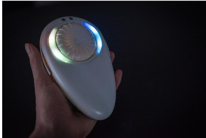
**Figure 2** A personal, portable light controller that we call Bolb (design by Remco Magielse, TU/e ID).
