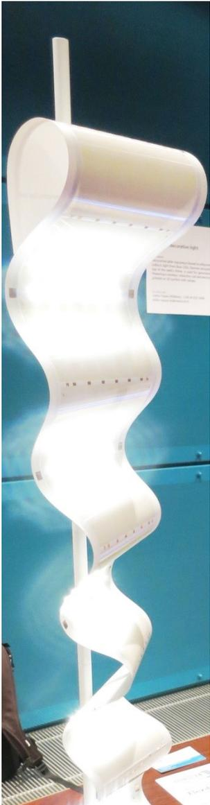
Figure 1 Flexible LED luminaire concept
